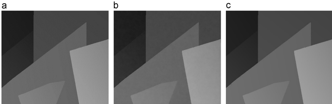
Fig. 1. The upsampling results of Eqs. (8) and (10). (a) Is the ground truth, (b) demonstrates the 8X upsampling result of Eq. (8), (c) shows the 8X upsampling result of Eq. (10). Compared (c) with (b), we can observe that there are nasty artifacts on the depth surfaces of (b).
