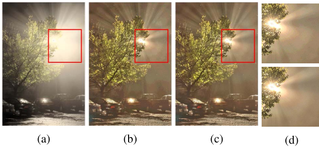
Fig. 8. Quantization artifacts demonstration. (a) Input HDR image (32 bit float, displayed by linear scaling). (b) Compressed image using 32 PBFIC (32 bins). (c) Compressed image using our method. (d) Zoom-in of the square in (b) as the upper image and that in (c) as the lower one.
